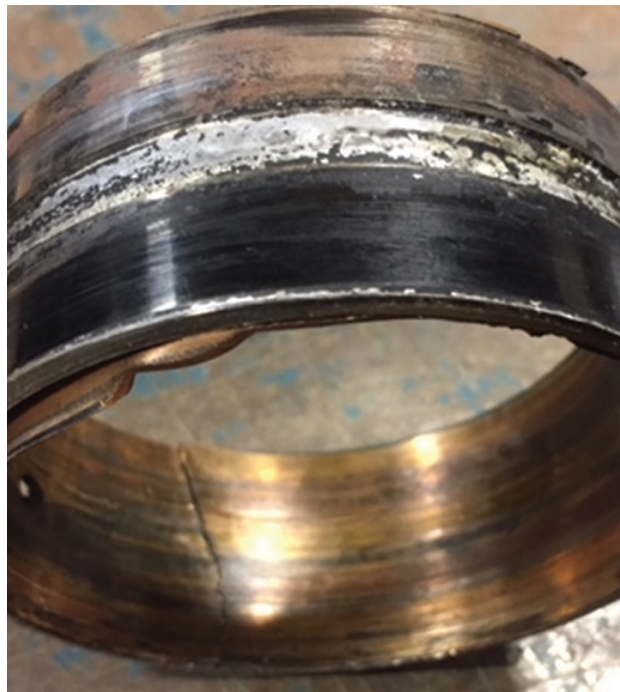
Failed Cam Bearing From Dry Start-Up
