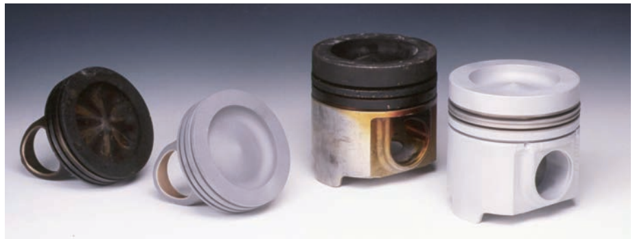
Photos on this page show before and after being blasted with soda. Courtesy ARMEC.
