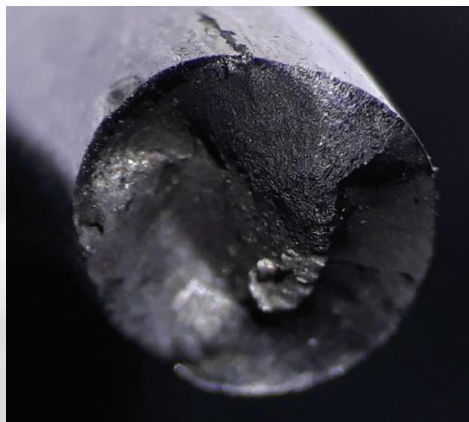
Figures 3 and 4: Broken wire surface defect and cross section.
