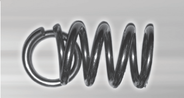
Figure 2: Broken valve spring.
