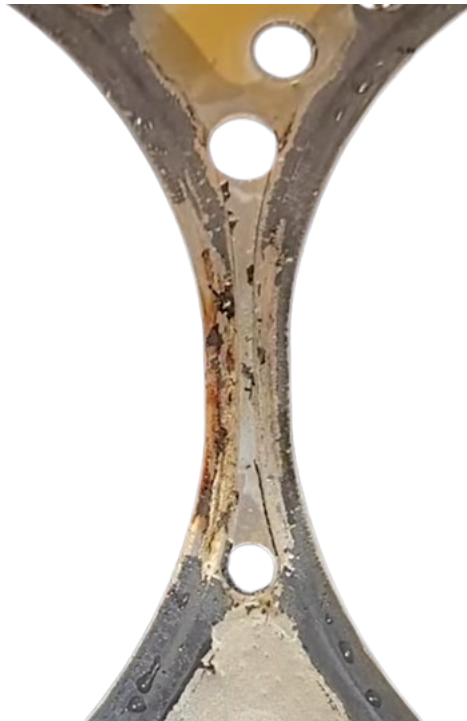
Figure 3: Failed Head Gasket
