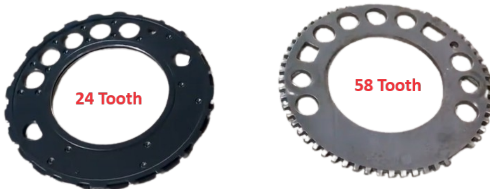
Figure 1: Comparison of 24X vs 58X Tooth Reluctor Wheels
