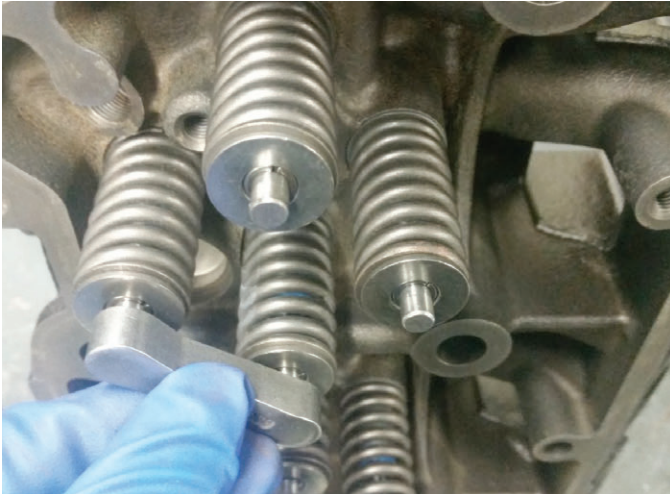
Final Inspection for Rocker Bridge Fitment
