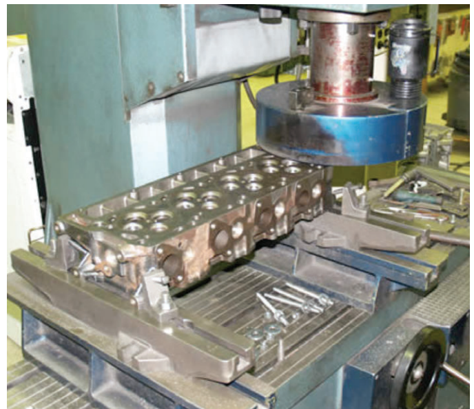
Milling the deck surface flat.
