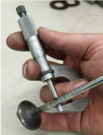
Qualifying valve stem for reuse, left; qualifying valve spring for reuse, right.
