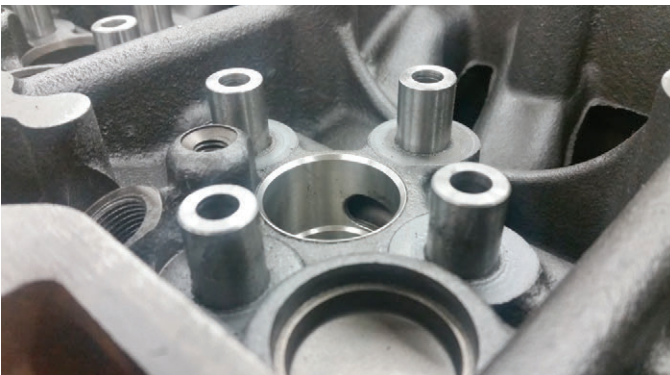
Injector Hole Sleeve - Post Installation
