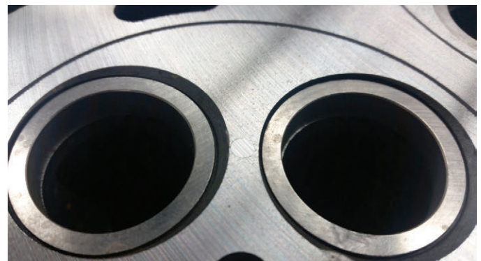
Lock-N-Stitch Repair Pin After Resurfacing
