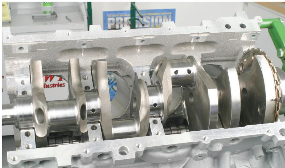
ABOVE: The tone wheel is positioned on the crankshaft with the two "arrowhead" shaped holes at 90° to the number 1/2 rod pin, with the series of large holes in the wheel positioned opposite from the first rod pin. That's only a rough description. DO NOT attempt to install a tone wheel by eyesight. It is absolutely critical to use the proper installation tool.
