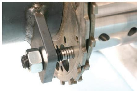
Here we see the installer tool's outer dowel pin engaged into the tone wheel's 8mm indexing hole.
