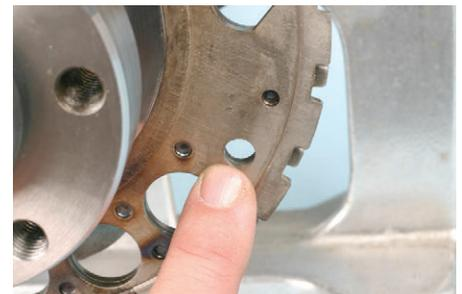
A closeup view of the tone wheel's indexing hole.
