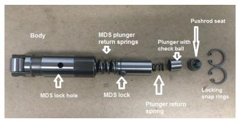
• In the normal mode, the MDS lock will be engaged into the MDS lock groove of the body
