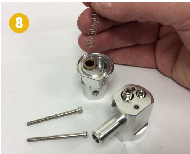
Figure 8: Removing spring to run in fixed orifice mode. Adjustability and backfire protection are maintained in fixed orifice mode.
