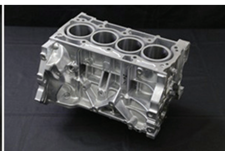
Left) A cast iron liner and conventional four-cylinder engine. (Right) A new type of four-cylinder engine with mirror bore coating. Courtesy Nissan Motor Company.
