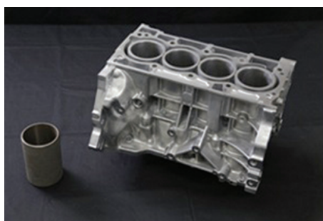
Left) A cast iron liner and conventional four-cylinder engine. (Right) A new type of four-cylinder engine with mirror bore coating. Courtesy Nissan Motor Company.
