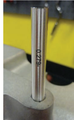
Determining hole ID with a gage pin. We use the go-no-go method for sizing small holes.
