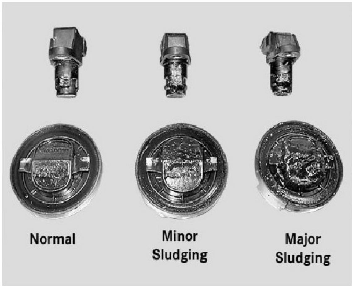
**Figure 1. The 3 Levels of Oil Sludge**
