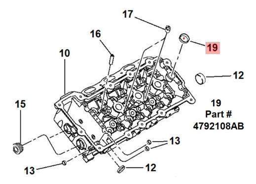
This vented plug Part #4792108AB is available from Dodge or Chrysler dealers. Some aftermarket core plug kits do not include the vented plug and drilling a hole the proper size is not an easy task because of its small size.
