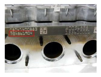
The cylinder head must be identified by the casting number highlighted in the illustration above. The casting number is located above the Cylinder 3 exhaust port. This is not the part number of the cylinder head. The part number and the casting number will differ.
