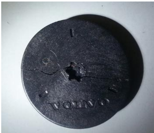
Figure 1. Cracked VVT Pulley Plug
