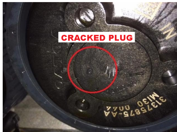
Figure 2. Cracked Plug in Pulley
