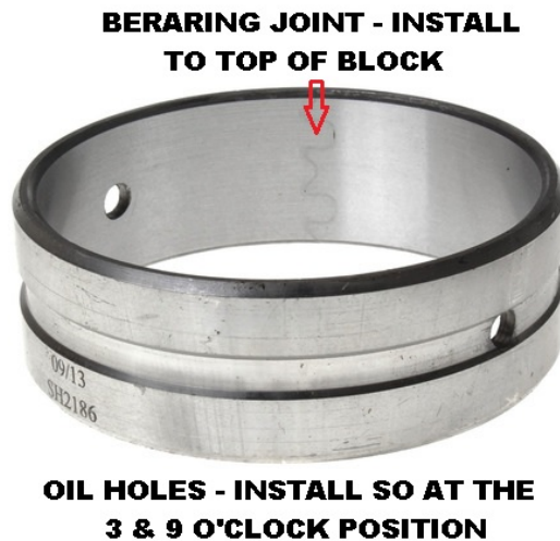
FIGURE 1. Identifying Camshaft Bearings Installation Direction
