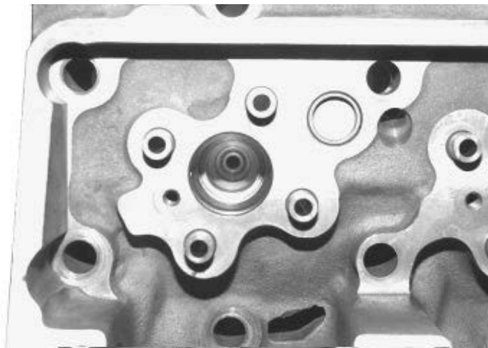
Properly Installed Injector Sleeve
