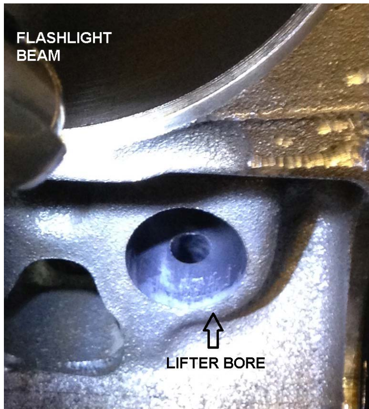
Figure 1. Lower Lifter Bore Wear
