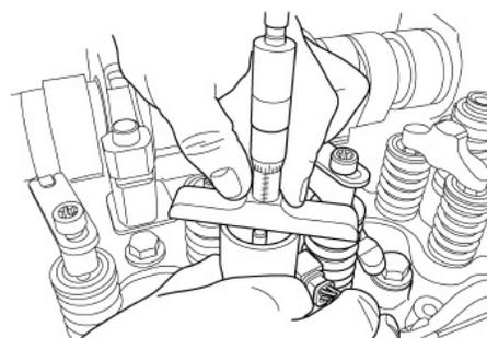
**Figure 2. Measuring Valve Stem Height**
