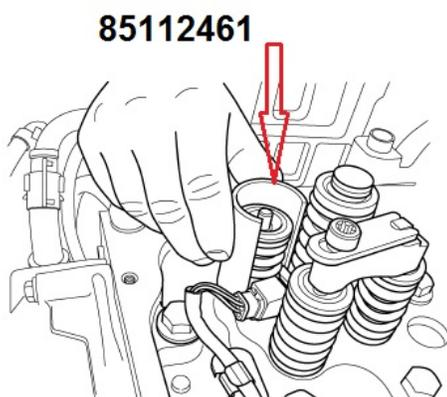
**Figure 1. Valve Stem Tool 85112461**
