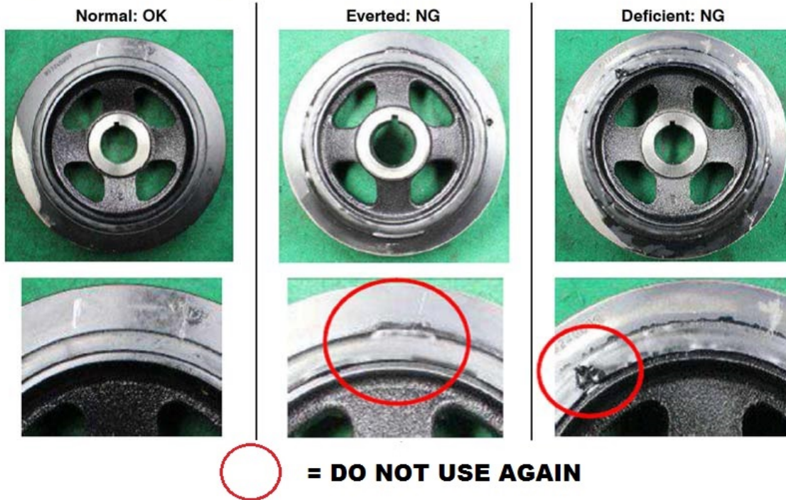
Figure 2. Crankshaft Pulley Re-Use Photos
