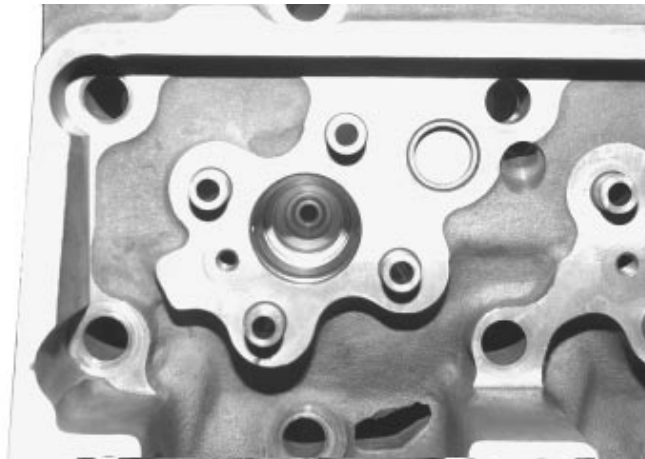
Properly Installed Injector Sleeve
